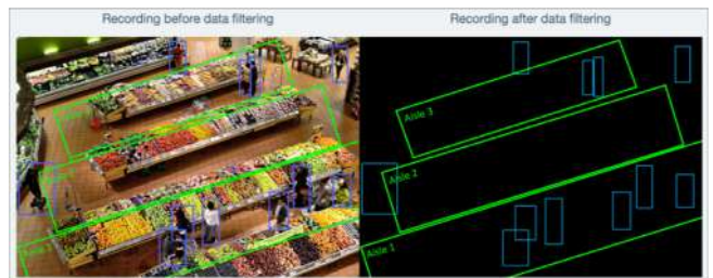
Figure 2: Surveillance footage without anonymization (left) and with vectorized streaming based anonymization (right)
